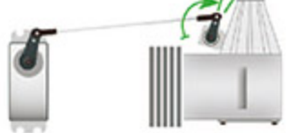
Move throttle to position at which the motor is just before to start running (electric heli) or idle position (nitro/gas heli) 移動油門到馬達開啓前的位置(電動直昇機)或油門怠速位置(引擎直昇機)
